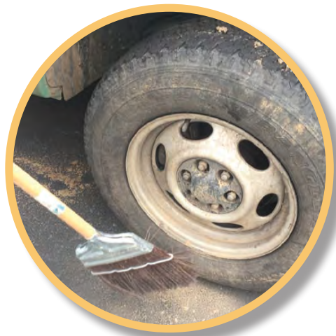
A stiff bristled broom can knock off mud clods as well as clean truck beds, wheel wells, and tires.
